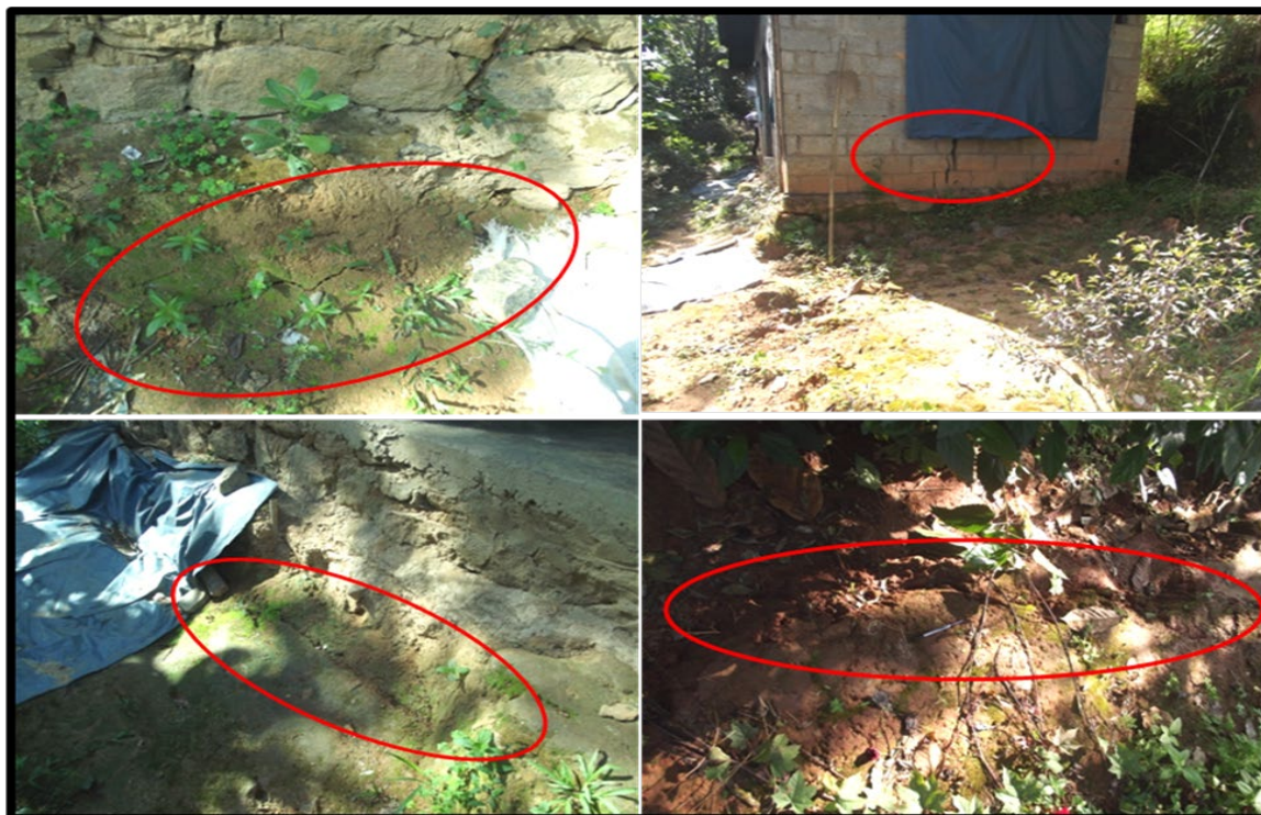
Fig. 5 Different segment of cracks developed near the crown of the landslide occurred at Kallarkutty junction
